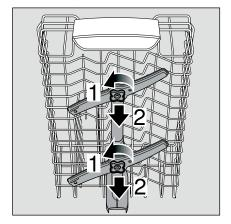
Remove the lower spray arm 24 upwards.
