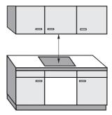
The safety distance specified by the manufacturer of the cooker hood must be maintained between the hob and the cooker hood above it.
